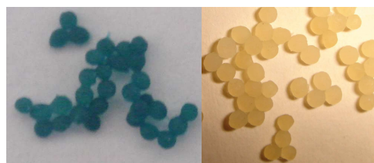
Figure 4 The hybrid microspheres (HCPL1.10) after the adsorption of Cu(II) (left) and after metal desorption (right); microparticle size is around 800 \mu m, by ESEM
