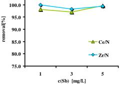
**Figure 2** Effect of concentration of Sb(III) in the feed solution on the distribution coefficient; pH = 6,  $c(CI, SO_4^{2-}) = 100 \text{ mg/L}$
