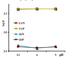
**Figure 1** Effect of pH on the distribution coefficient; c(Sb) = 5 mg/L,  $c(Cl^*, SO_4^{2^*}) = 100 \text{ mg/L}$
