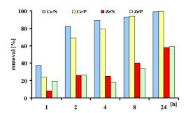
**Figure 3** Study of sorption kinetics; c(Sb) = 5 mg/L,  $c(Cl, SO_4^2) = 100 mg/L$ , pH = 6
