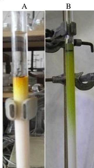
Figure 12 Comparison of color ion-exchange columns after sorption \text{Cr}^{\text{VI}} . A - resin with trimethylammonium functional groups, B - resin with aminomethylglucitol functional groups
